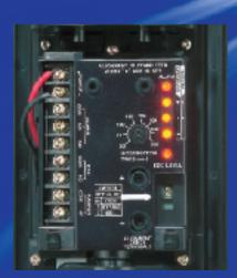
LED Level Meter for Beam Alignment Three LEDs on the receiver act as a Level Meter to visually display the beam reception level.
