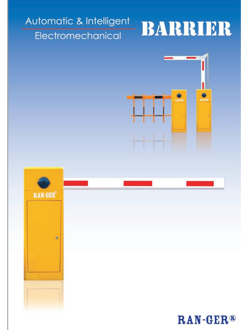
The Chassis is manufactured from 14 gauge zinc plated sheet steel onto a base frame of stainless steel, then finished with epoxy powder coating paint for maximum protection against corrosion. The boom arm uses a special aluminum material with red reflective tape for clear night vision.
